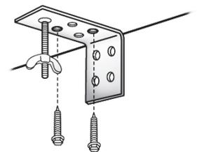
OPTION: Mounting in the ceiling or inside the window opening
